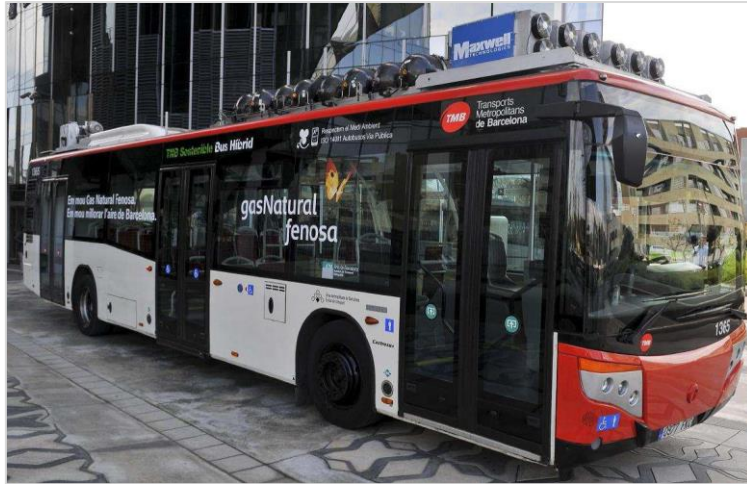
Retrofitted CNG bus transformed into a hybrid vehicle (picture: courtesy of TMB)
